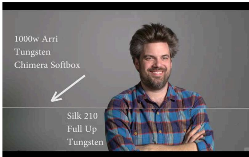
Before I did this test, I would never have thought that the Silk 210 would be a real-world replacement for my 1K tungsten fixtures. Discoveries like this are why I wanted to do the real-world test. A big surprise for me was how we got such matching results despite the fact that the face of the Silk 210 is so much smaller than the Chimera softbox.
